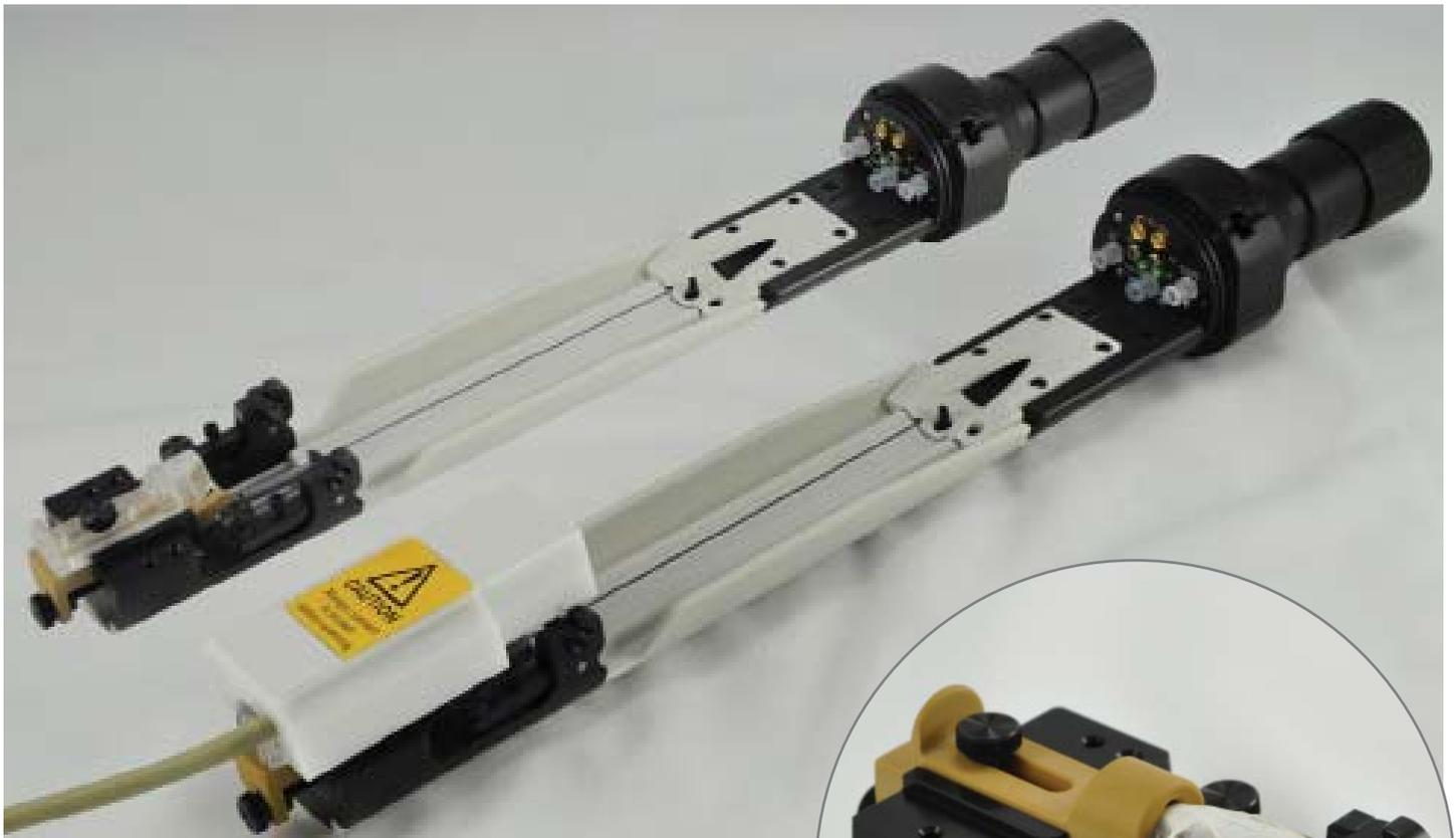
**Stereotaxic Ear System** with conventional a-traumatic ear bars, that are drill to accept handle extensions. The ear bar handle extension facilitates the loading of the animal into the headstock area, and are removed to allow small bore insertions. The headstock area is pre-configured to supply anesthesia gas directly to the animal. The design also provides for a EVAC curcuit to remove used gases from the area.
